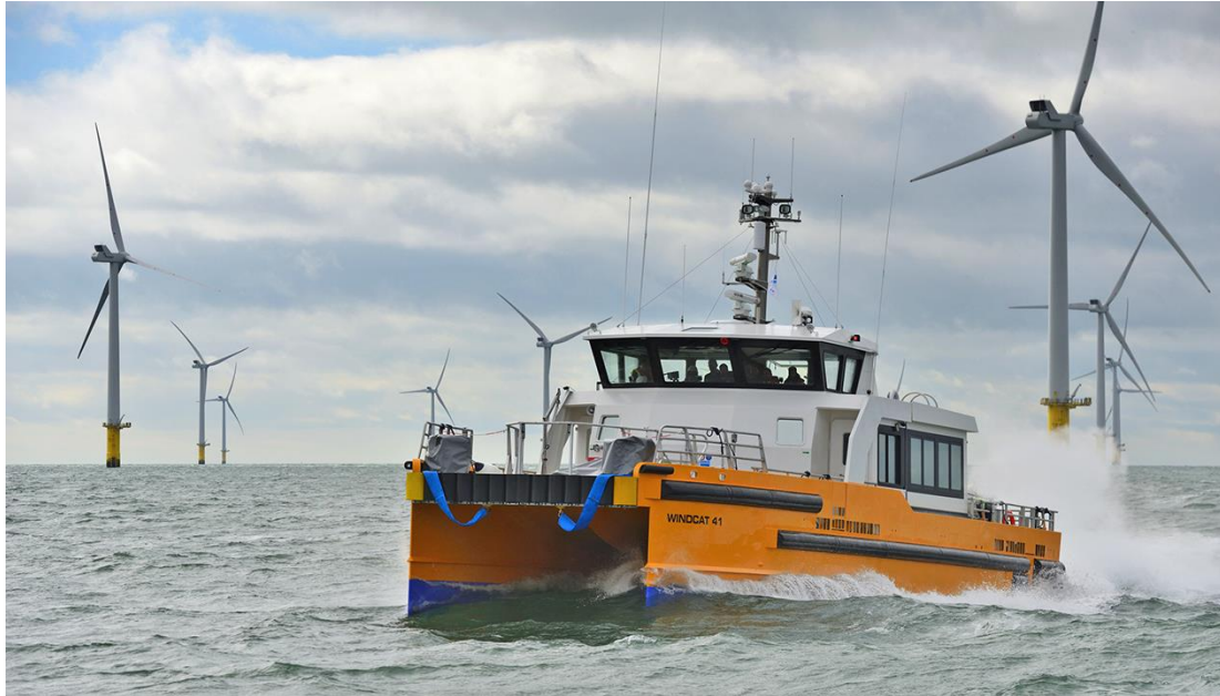
Graphic 4-25 Typical crew transfer vessel which can carry 12 to 16 passengers and equipment.
