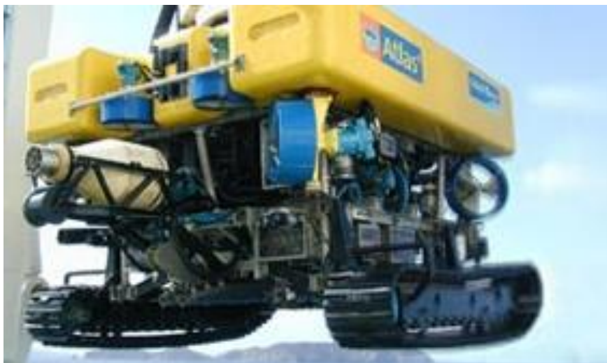
Graphic 4-16 Typical marine cable jetting seabed fluidiser
