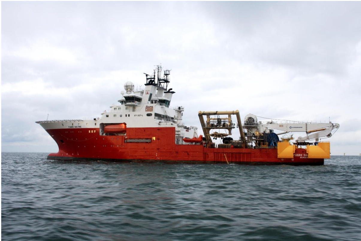
Graphic 4-15 Example array cable installation vessel (Rampion 1 offshore wind farm)
